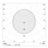
Correlated color temperature: 6000 kelvin Rated median useful life: 50000h L70 at 25°C Luminaire input power: 15 w
