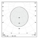
Correlated color temperature: 3000 kelvin Rated median useful life: 50000h L70 at 25°C Luminaire input power: 24 w
