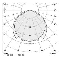
Correlated color temperature: 3000 kelvin Rated median useful life: 50000h L70 at 25°C Luminaire input power: 19.2 w
