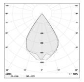
Correlated color temperature: 3000 kelvin Rated median useful life: 50000h L70 at 25°C Luminaire input power: 100 w
