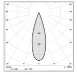
Correlated color temperature: 3000 kelvin Rated median useful life: 50000h L70 at 25°C Luminaire input power: 2x35 w
