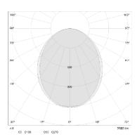
Correlated color temperature: 6000 kelvin Rated median useful life: 50000h L70 at 25°C Luminaire input power: 19.2 w
